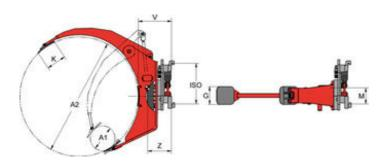
Short arm fixed - 2 hydraulic functions, Especially designed for extreme narrow rolls (width from 150 mm)
