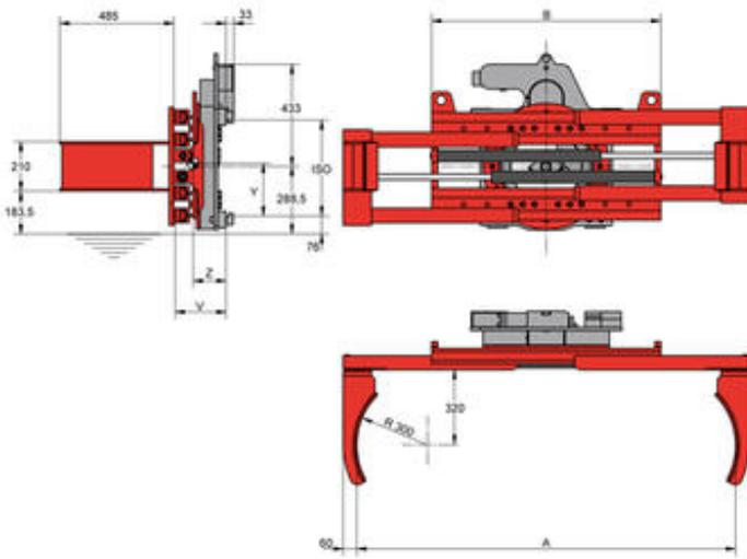
360° rotation continuous - to transport cylindrical steel drums - arms covered with Remagrip, 2 hydraulic functions
