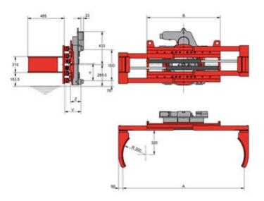
360° rotation continuous - to transport cylindrical steel drums - arms covered with Remagrip, 2 hydraulic functions
