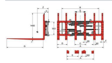
with independent sideshift - with bolt-on forks, Pallet handling lengthwise  $800 \times 1.200 \text{ mm}$  for 4 or 6 pallets - 2 hydraulic functions
