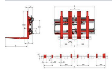
with independent sideshift - for 2 or 4 pallets side by side or 4 or 8 pallets - 2 hydraulic functions
