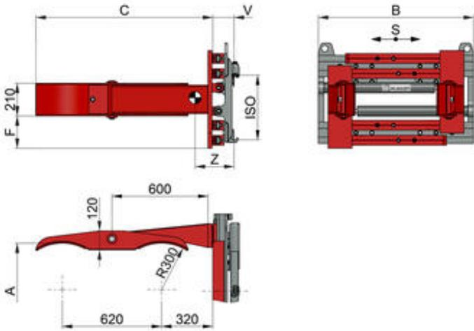
with independent sideshift - for cylindrical steel drums - 2 hydraulic functions, This Drum Clamp can transport 2 or 4 drums palletless and safely.
