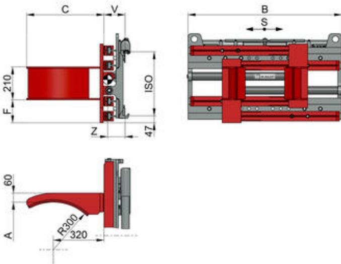
with independent sideshift - for cylindrical steel drums - 2 hydraulic functions, This Drum Clamp can transport 1 or 2 drums palletless and safely.
