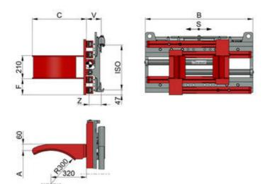
with independent sideshift - for cylindrical steel drums - 2 hydraulic functions, This Drum Clamp can transport 1 or 2 drums palletless and safely.
