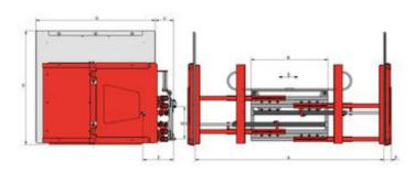
with independent sideshift - rubber coated - both arms swivelling - 2 hydraulic functions
