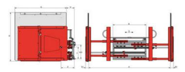
with independent sideshift - rubber coated arms - one arm fix, one arm swivelling - 2 hydraulic functions
