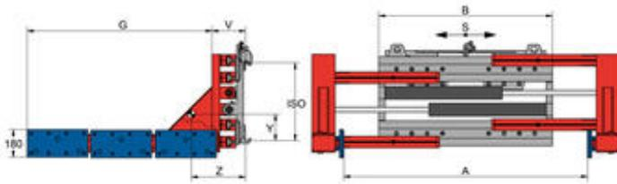
with independent sideshift - with mechanical equilibration plates with Vulcollan coating - 2 hydraulic functions
