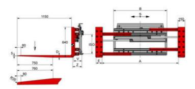
with independent / valveblock sideshift - 2 hydraulic functions - with bolt-on forks - fork length 1.150 mm
