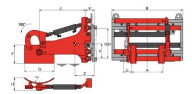
without sideshift - with hydraulically tiltable clamp arms 180° forward - 2 hydraulic functions
