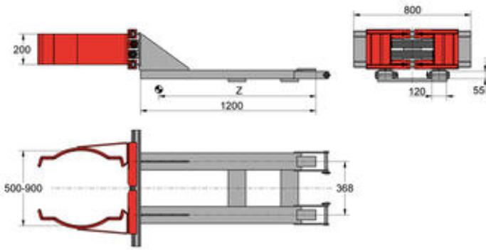
slip-on-fork version, arms coated with Remagrip - for cylindrical steel drums and garbage bins - without rotation - 1 hydraulic function
