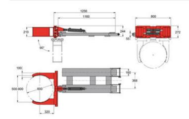
slip-on-fork version, arms coated with Remagrip for cylindrical steel drums - without rotation - 90° forward tipping - 2 hydraulic functions
