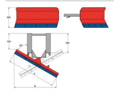
mechanically tiltable - to clear to right or left side - with fork pockets for slipping on forks with a maximum fork cross cut, of  $160 \times 60 \text{ mm}$  - distance between fork pockets measured over the outer edges 560 mm
