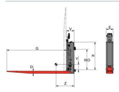
for mounting on ISO fork carriage - hydraulically foldable - 1 hydraulic function
