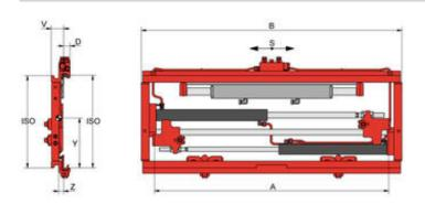
with independent sideshift - without forks - for forks acc. to ISO 2330 - 2 hydraulic functions
