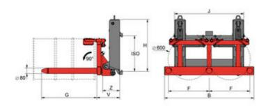
90° tipping, rubber coated flaps - for cylindrical steel drums - 2 hydraulic functions
