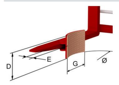
slip-on version, for handling of cylindrical steel drums) - rubber coated
