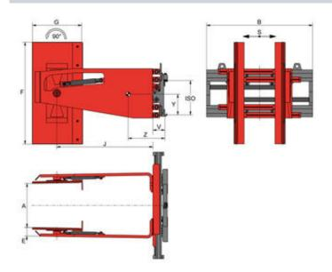
with independent sideshift - rubber coated arms - both arms 90° forward tipping - 2 hydraulic functions + solenoid valve
