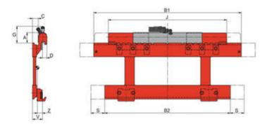
1 hydraulic function, Quick mounting, hook-on type, end-of-stroke slow-down SOFTSTOP, high visibility design, e.g. CofG up to 1.800 mm, Bottom brackets with roller guidance, SMOOTHROLL.
